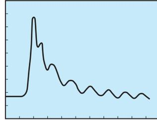
The R12290U and R1328U are built in a special metal housing designed with well considerations of electrode shape, housing shape, the widening of bandwidth and the impedance matching of a load resistance output connector. Their laser pulses are thus output through the N-R connector of an excellent frequency characteristic. For this reason, you must use their output cable, connector and characteristic impedance of the measuring system at 50 Ω.
