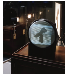
The Japanese character for “i” displayed on a cathode-ray tube (The device in the photograph is a reproduction)
