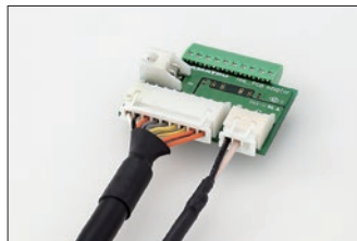
Connection example with A11134-08(-09) and -10(-11)
