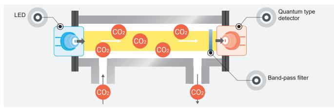
Since there is a  $CO_2$  absorption band near the wavelength of 4.3 µm, light is absorbed by  $CO_2$  when exposed to light in that wavelength region. The amount of light absorbed increases as the  $CO_2$  concentration increases, and the  $CO_2$  concentration can be measured from the change in the signal level of the photosensor due to changes in the amount of light absorption.
