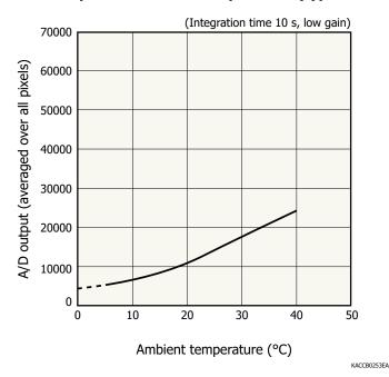
$\mbox{\ensuremath{A/D}}$  output is the sum of the sensor and circuit offset outputs and the sensor dark output.
