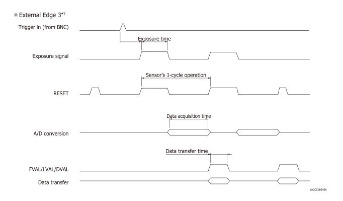
\*7: Data of multiple lines can be acquired with a single external trigger signal as wall as similar operation to External Edge 1.
