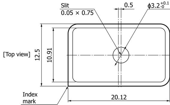
**Enlarged view of slit (unit: mm)**
