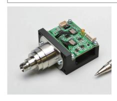
C14076-01 is an optical measurement module that can detect low-level light. It contains a thermoelectric cooled single photon avalanche diode (SPAD). The C14076-01 has nearly the same functions as the C13001-01. Since this product is compact and lightweight, it is suitable for integration into equipment. The C14076-01 requires heat dissipation.
