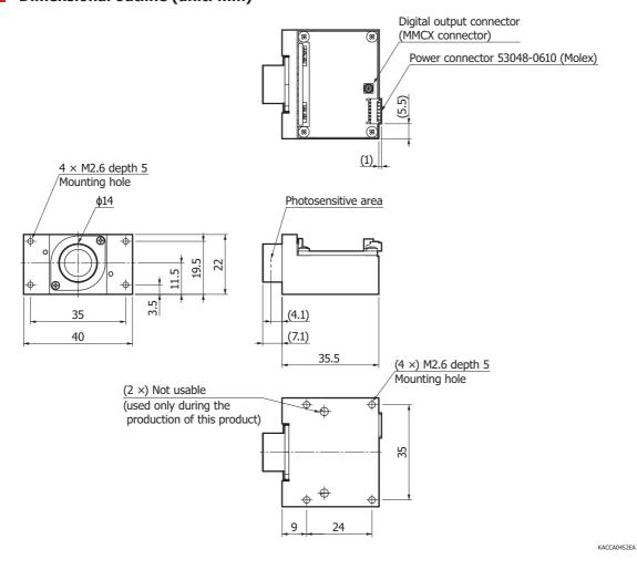
Note: When using this product, provide heat dissipation measures by using heatsinks or through thermal coupling with the enclosure that you will use. Keep the thermal resistance to 3 °C/W or less.
