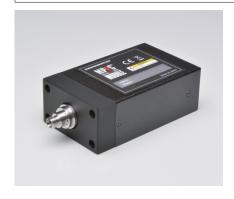
The C13001-01 is a module for evaluating fiber coupling type single photon avalanche diode (SPAD). This module consists of a fiber coupling type (SPAD), an amplifier, a comparator, a SPAD bias circuit, and a temperature controller. The module operates by simply connecting to an external power supply (±5 V). The C13001-01 series has nearly the same functions as the C14076-01. Note that the C13001-01 does not require heat dissipation measures.
