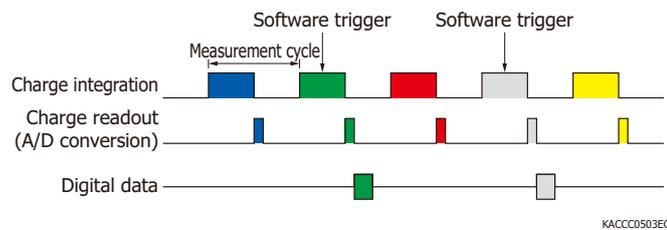
**(2) Synchronous data measurement at software trigger input**
