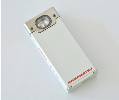
These are compact modules with built-in MEMS-FPI spectroscopic sensors, light sources, and control circuits. Since they come with evaluation software that has functions such as setting measurement conditions, data acquisition and storage, and graph display, spectrum and absorbance can be easily measured by connecting to a PC via USB. It can also be used to characterize MEMS-FPI spectroscopic sensors C14272, C13272-03, and C14273.
