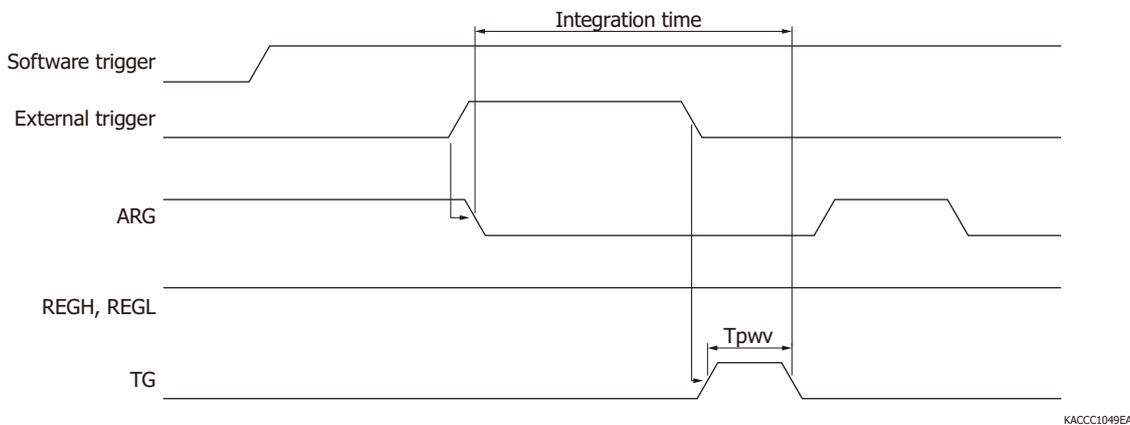
In this mode, sensor integration starts at the timing when an external trigger is input. External triggers input before software triggers are input are ignored. Integration time is set according to the pulse width of the external trigger. Integration time = Pulse width of external trigger + Tpw
