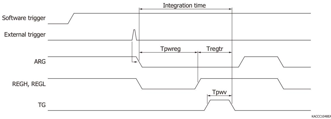
In this mode, sensor integration starts at the timing when an external trigger is input. External triggers input before software triggers are input are ignored. The integration time is set using application software.
