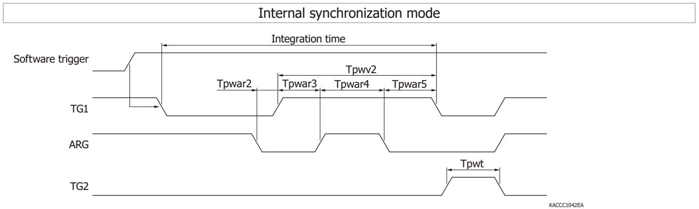
In this mode, sensor integration starts at the timing when a software trigger is input. The integration time is set using application software.
