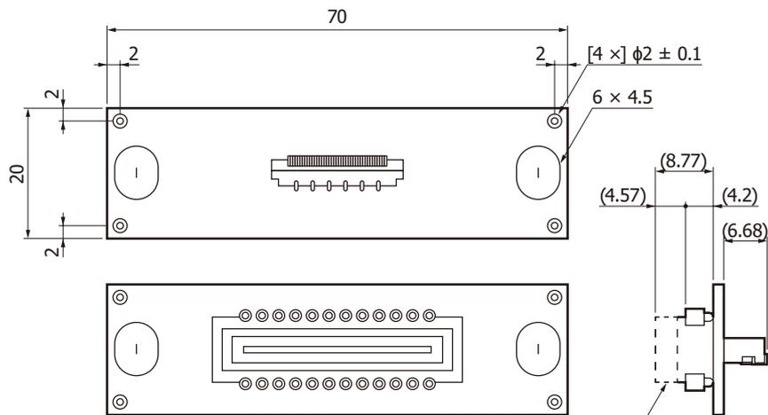
Broken line: When sensor attached
