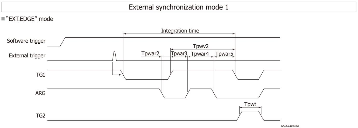
In this mode, sensor integration starts at the timing when an external trigger is input. External triggers input before software triggers are input are ignored. The integration time is set using application software.
