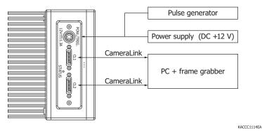
$\cdot$  Connect the power cable according to the pin arrangement.
