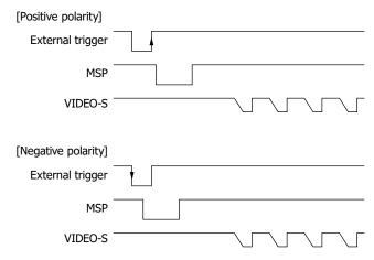
Delay time from when an external trigger is input to when exposure is started=30 ns  $Jitter=\pm10$  ns
