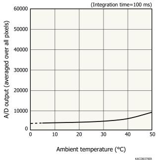
A/D output is the sum of the sensor and circuit offset outputs and the sensor dark output.
