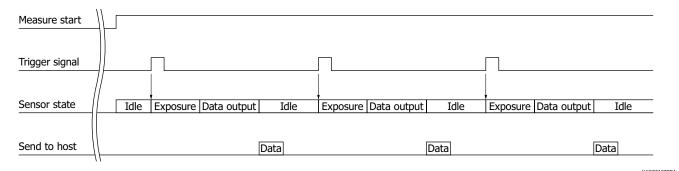
(2) Data measurement at external trigger input
