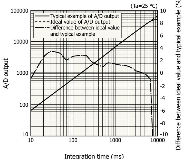
A/D output is the output with dark output is subtracted when light is input. The difference between the ideal value and typical example contains a measurement error. The smaller the A/D output, the larger the measurement error.
