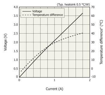
\* Temperature difference between photosensitive area and package heat dissipation area
