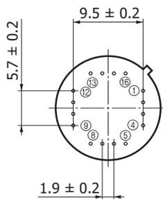
Position accuracy of photosensitive area center with respect to cap center
