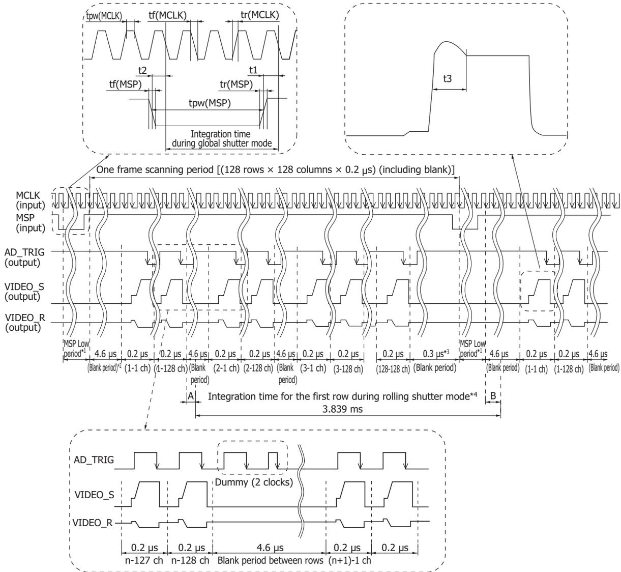
\*1: The minimum number of MCLK pulses during the MSP low period is 20. The integration time can be changed by adjusting the MSP low period.
