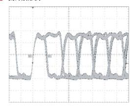
縦軸: 30 mV/div.、横軸: 5 ns/div. (Ta=25 °C, Vcc=5.00 V, R1=100  $\Omega$ , R2=300  $\Omega$ , CL=20 pF)
