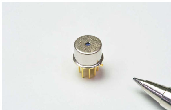
[Figure 1-2] MEMS-FPI spectrum sensor
