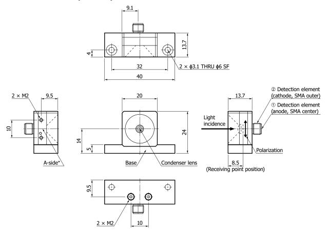
\* A-side can be fixed on the base as the bottom aspect. Tolerance unless otherwise noted: ±0.3 Both ① and ② are electrically insulated from the package.
