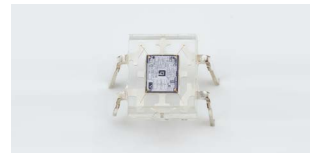
DIP (Dual Inline Package)
