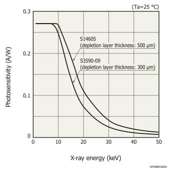
Photosensitivity vs. X-ray energy (theoretical value)
