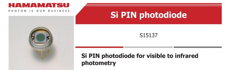
The S15137 is a Si PIN photodiode developed for YAG lasers (1.06  $\mu$ m). The photosensitivity at 1.06  $\mu$ m is 0.57 A/W (typ.), which is about 1.5 times higher than that of previous products. The PIN structure allows high-speed response and low capacitance. The photosensitive area is as large as  $\phi$ 5 mm, making optical axis alignment easier.
