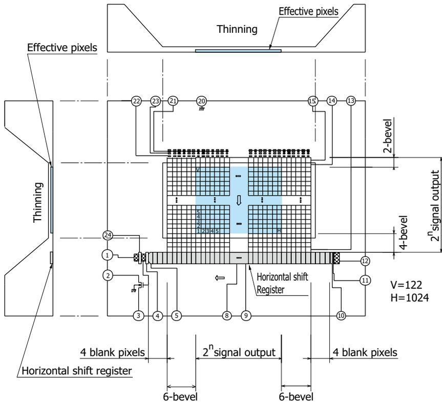
Note: When viewed from the light input side, the horizontal shift register is covered by the thick area of the silicon (insensitive area), but long-wavelength light may pass through the insensitive silicon area. This light may be received by the horizontal shift register. Take measures such as shielding the light.
