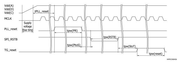
Note: At power-on, input the SPI\_RSTB and Reset signals at the timings shown in the figure above to initialize the timing circuit and SPI circuit after all the supply voltages have risen to the recommended operating conditions [Vdd(A)=Vdd(D)=3.0 V, Vdd(C)=2.4 V].
