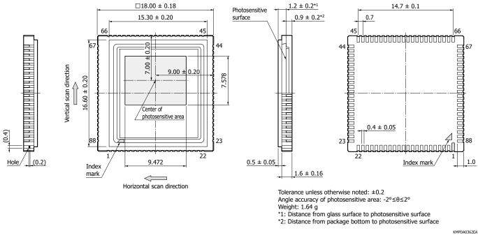
Note: There is a hole on the side of this product that allows outside air to enter the package to prevent condensation. Do not wash the product by soaking in cleaning solution, as the solution will enter the package and may cause problems.
