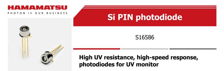
The S16586 is a high-speed response Si PIN photodiode that has achieved high reliability for monitoring ultraviolet light. They exhibit low sensitivity deterioration under UV light irradiation and are suitable for applications such as monitoring intense UV light sources.
