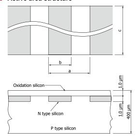
S3901-1024Q: a=50 μm, b=45 μm, c=2.5 mm S3904-2048Q: a=25 µm, b=20 µm, c=2.5 mm
