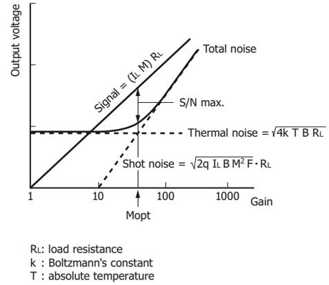
In this case, the optimum gain (M<sub>opt</sub>) is obtained under the conditions that maximize the S/N described in equation (2-4). If Ids can be ignored, the optimum gain is given by equation (2-6).
