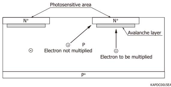
[Figure 2-10] Crosstalk (S8550-02, element gap: 0.7 mm, typical example)
