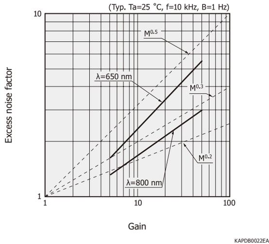
The excess noise factor (F) can also be approximated as  $F=M^x$  (x: excess noise index) because the equation for shot noise can be expressed in the form of  $I_n^2=2q I_L B M^{2+x}$ . As explained, APDs generate noise due to the multiplication process, so excess noise increases as the gain becomes higher. On the other hand, the signal is also increased according to the gain, so there is a gain at which the S/N is maximized. The S/N for an APD can be expressed by equation (2-4).
