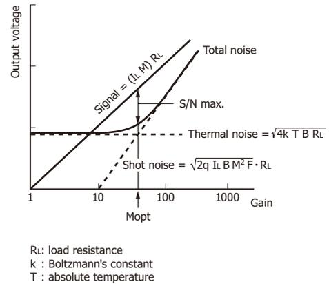
In this case, the optimum gain ( $M_{opt}$ ) is obtained under the conditions that maximize the S/N described in equation (2-4). If  $I_{ds}$  can be ignored, the optimum gain is given by equation (2-6).
