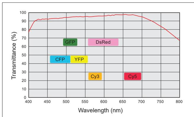
Spectral transmittance (in bypass mode)
