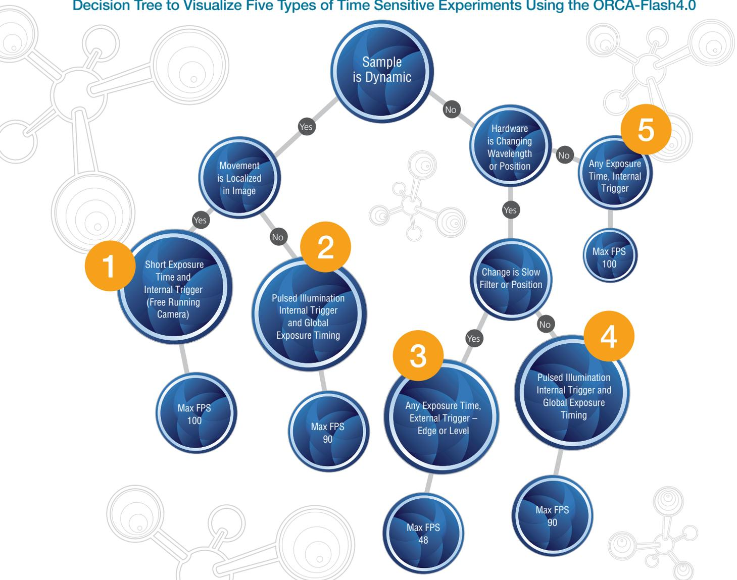
Maximum frame rates are shown for full resolution (2048 x 2048) images on an ORCA-Flash4.0 V2 using the Camera Link data transfer interface and a 1 ms exposure. In experiment 3, a hardware change of 10 ms was used. In experiments 2 and 4, a minimum Global Exposure Timing setting of 10 microseconds is possible which would result in a maximum rate of 99.9 FPS.
