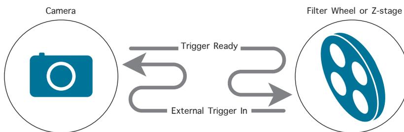
The filter wheel or z-motor tells the camera that it has stopped moving. The camera takes an image and tells the filter wheel or stage the image is captured and it is OK to move to the next position.
