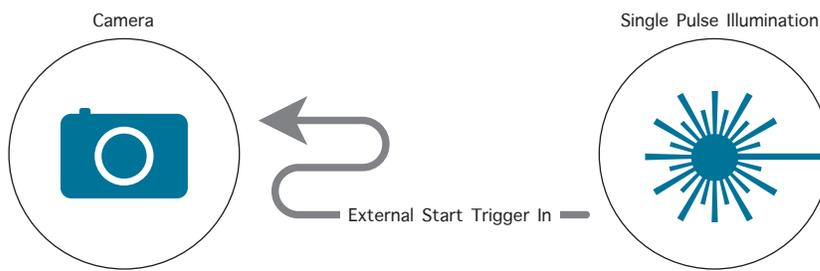
The illumination device triggers the camera to start image acquisition.
