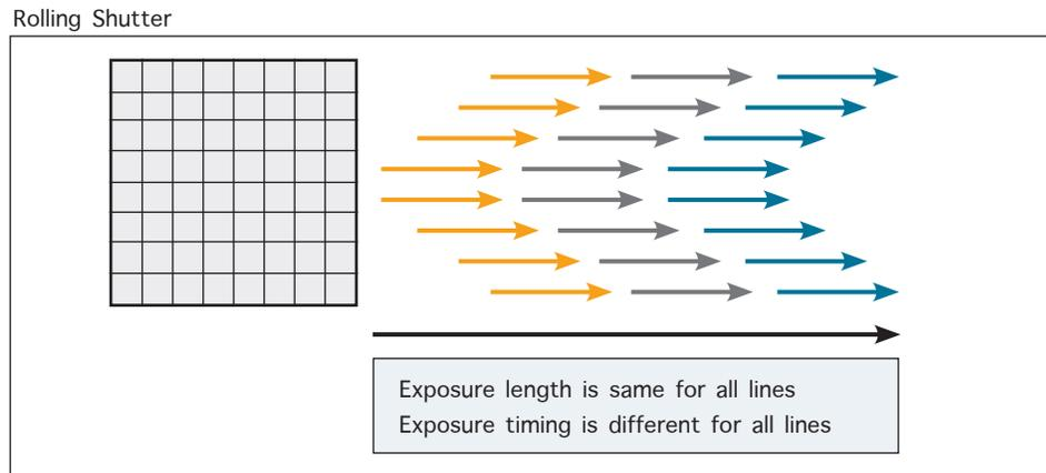
Figure 10-2 Readout timing of Rolling Shutter
