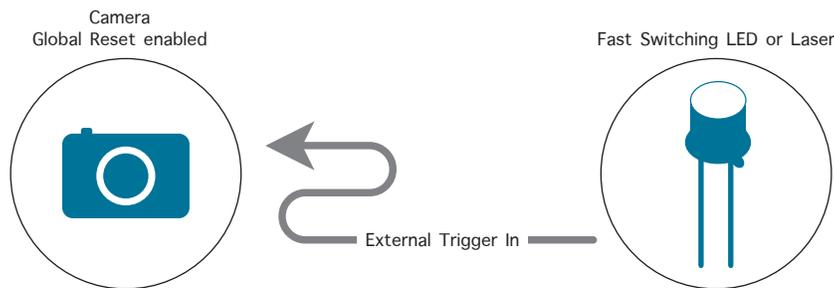
The pulsed illuminator triggers the camera to start acquiring an image and shines light on the sample only during the period when all lines on the sensor are available to be exposed simultaneously.
