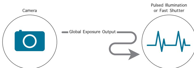
The camera sends a trigger signal to the shutter or pulsed illumination.
