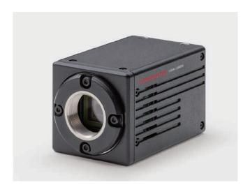
The C16741-40U is an InGaAs camera with sensitivity in the visible to near infrared region from 400 nm to 1700 nm. It has a USB 3.1 Gen 1 interface port which supports 12 bit image acquisition and exposure time adjustment. This makes the C16741-40U ideal for use in a wide range of applications including internal inspection of silicon wafers and devices, laser beam alignment and evaluation of solar cells.
