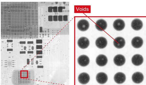
As bidirectional scanning is supported, the C12300 series can efficiently scan the entire surface of PCBs mounted with electronic components, and can inspect voids in solder at high resolution.
