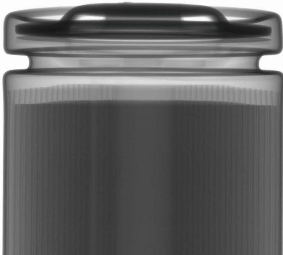
X-ray image of cylindrical lithium-ion battery (LiB)
