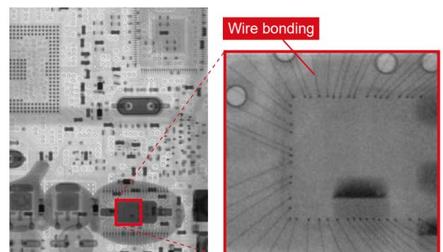
The C12300-323 is compatible with tube voltages up to a maximum of 180 kV. It is capable of transmitting X-rays through heat sinks and other metal parts to inspect for defects in wire bonding on PCBs.
