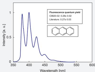
The quantum yields of fluorescence standard solutions were measured with our Absolute PL quantum yield measurement system. The fluorescence standard solutions have been used for determining PL quantum yield based on a relative method. For the most compounds, the quantum yield measured by our system shows excellent agreement with the values given in the literature, proving the high reliability of our system.
