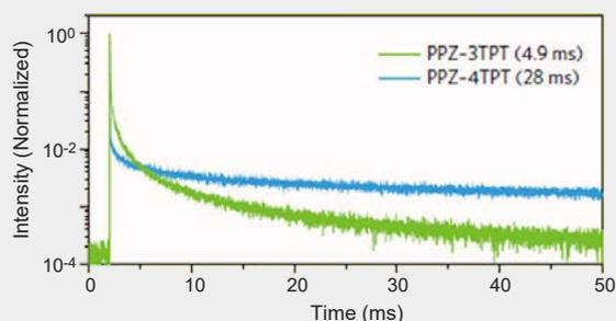
Delayed fluorescence of TADF material results in that small gap of  $\Delta E_{st}$ , which is defined as the energy gap of  $S_1$  state and  $T_1$  state, is in the microsecond range. On the other hand, wide gap of  $\Delta E_{st}$  is in millisecond range.
