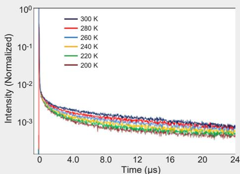
Temperature dependence of transient PL decays of triarylboron-based OLED emitter doped in CBP (16 wt%).
