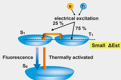
TADF (Thermally activated delayed fluorescence) is known well as the 3rd generation OLED material which is high efficiency and cost saving, furthermore can be replaced with phosphorescence material. The data shows the example of fluorescence lifetime measurement of blue TADF material. In order to achieve the high efficiency, the molecule design is the important factor to minimize the energy gap of excited singlet state ( $S_1$ ) and excited triplet state ( $T_1$ ).
