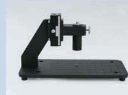
This stage accommodates samples up to  $\Phi 200$  mm in diameter. It comes with a visible light condenser lens with corrected chromatic aberration.
