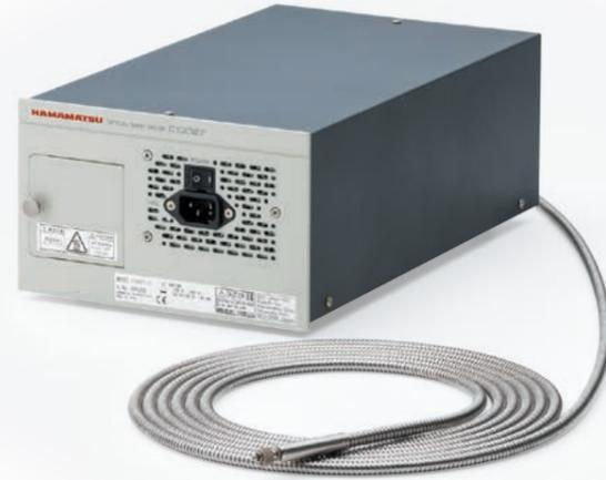
**Measurable range** **Glass:** 10 nm to 100 μm
