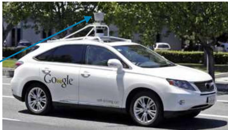
Velodyne LiDAR system: 64 channels (beams) 905 nm,  $1.3$  or  $2.2 \times 10^6$  points per second, 5 - 20 Hz rotation, APD photo-sensors.
