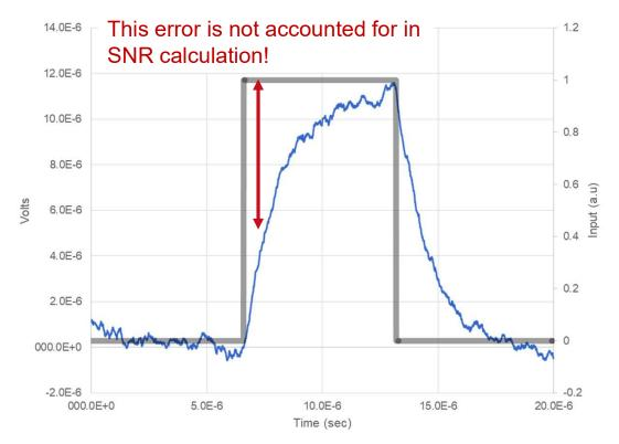
• Degradation can be caused by detector speed or readout circuit bandwidth and slew rate.
