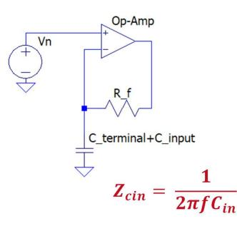
$$v_{out} = v_{Nrms} \left( 1 + \frac{R_f}{Z_{Cin}} \right)$$
