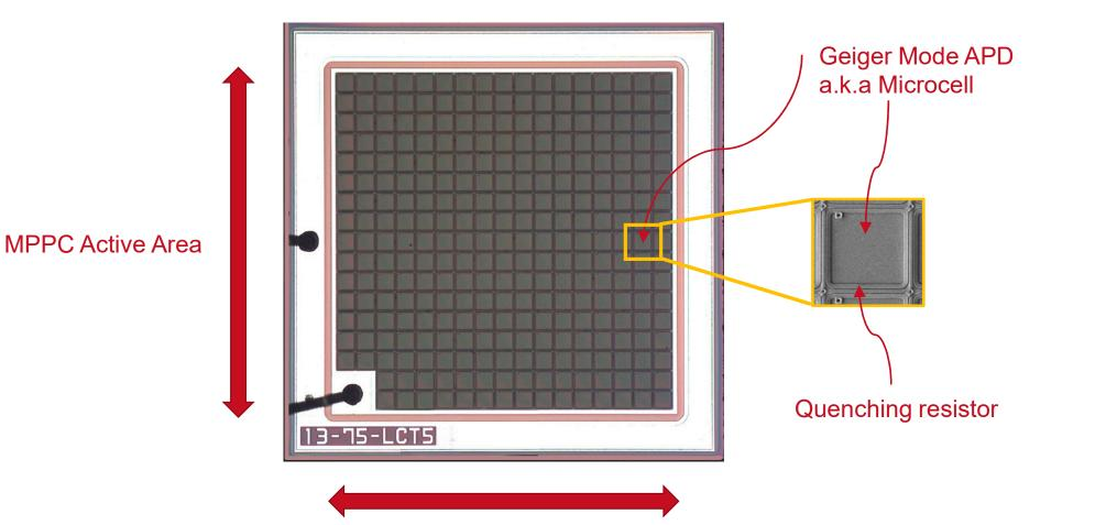
Cause of Excess Noise in MPPC (SiPM)
