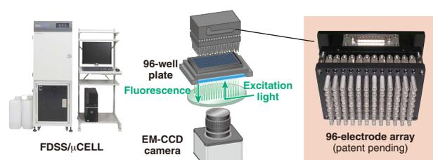
Our developed 96-channel electrode array is used coupled with the FDSS/ $\mu$ CELL. The electric field stimulations are given to all 96 wells in a microplate simultaneously by electrode array that is positioned at the upper side over the microplate. The excitation light is introduced from the bottom side, and fluorescence signals from cells are monitored with an EM-CCD camera.
