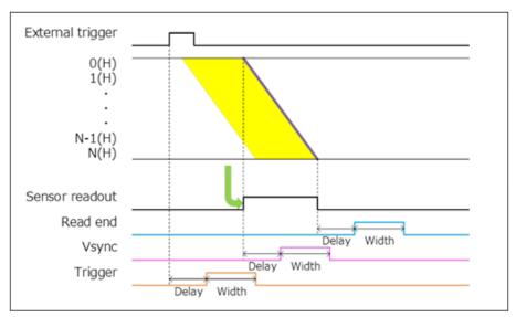
Figure 11-12 Programmable timing output
