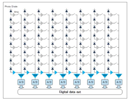
Figure 10-1 Structure of CMOS image sensor
