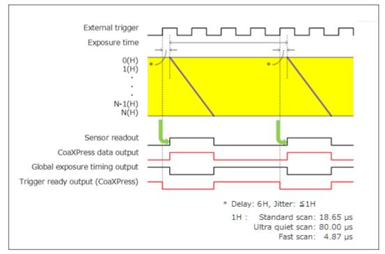
The following figure shows the exposure timing when the Trigger Times is set as 4.
