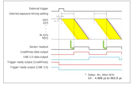
Figure 11-17 (Ex. rising edge, Top to bottom readout)
