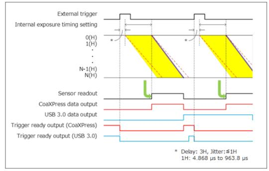
Figure 11-16 (Ex. rising edge, Top to bottom readout)
