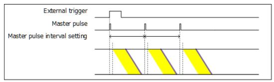
Figure 11-24 (Camera: Normal area, Edge trigger mode) (The number of pulses is specified as 3)
