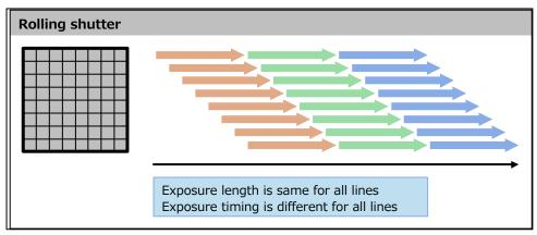
Figure 10-2 Readout timing of Rolling shutter
