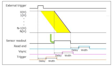
Figure 11-18 Programmable timing output (Top to bottom readout)
