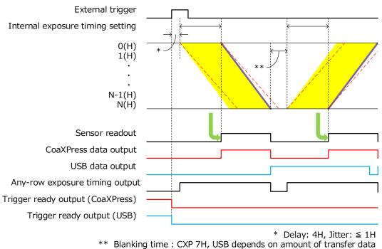
1H readout time : 7.309 μs – 233.9 μs
