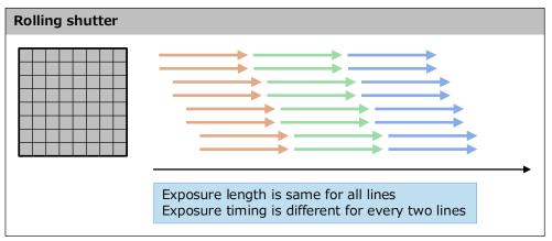
Figure 10-2 Readout timing of Rolling shutter
