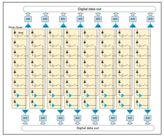
Figure 10-1 Structure of CMOS image sensor
