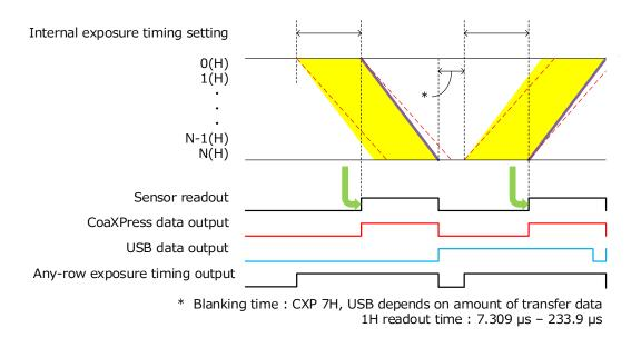
Figure 11-18 (Ex. Bidirectional readout)
