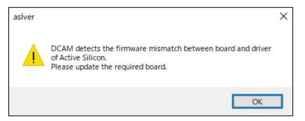
When this message is displayed, you need to update the firmware of the interface board to use the connected camera. In this case, an update procedure will be displayed on the screen when you click "OK". Update the interface board according to it.
