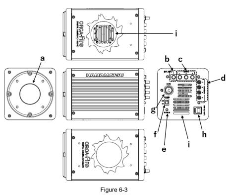
Place the camera the ventilation ports to be lateral side. Do not place the rear panel of the camera, which connectors are located, to be at the bottom (Do not block ventilation openings.).
