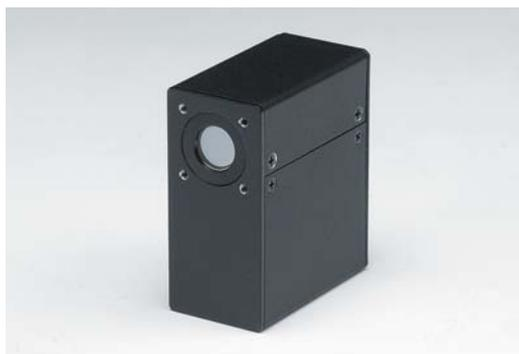
The H11890 series is a compact photon counting head consisting of a metal package photomultiplier tube along with a high speed photon counting circuit and a high-voltage power supply unit. The high voltage supply for the photomultiplier tube and the discriminator level are preset to optimum values, allowing photon counting measurement by just connecting to a PC.
