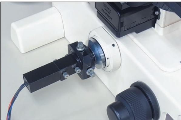
The A11027 is a holder block for mounting a pinhole. The screws can be used to adjust the pinhole's position in the XY directions. The built-in lens collimates the light that passes through the pinhole and converges the light on a photodetector.
