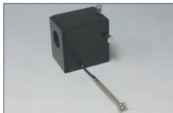
1. Remove the two cover screws using a Phillips-head screwdriver, and then remove the cover.
