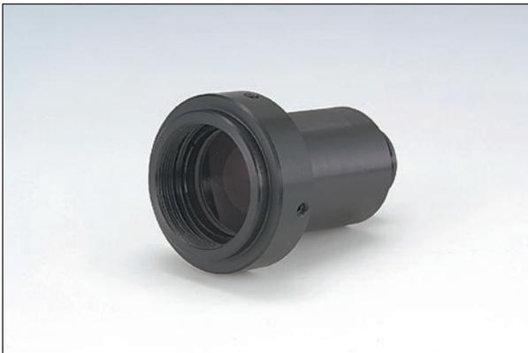
This block widens the diameter of a collimated beam of light to 2.5 times its original size or reduces the diameter to 1/2.5 times its original size. This block has a C-mount thread for connecting to another device.
