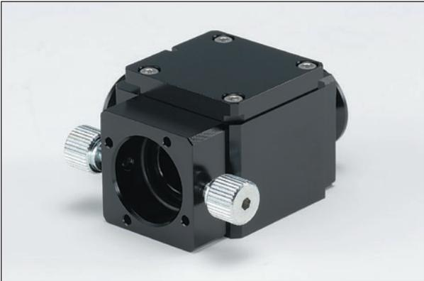
The A10035-90 is a holder block designed to hold a 15 mm cubic type beam splitter. There are M3 screw holes in the bottom of the block for holding.
