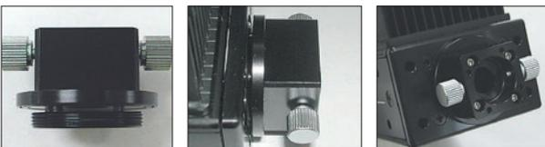
1. Loosen the four screws on the adapter block and make sure the C-mount ring is separated about 1 mm from the adapter block body.
