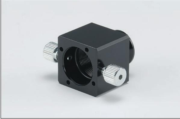
The A10033-90 is a holder block that allows you to insert an optical filter. The filter is held by the spacer ring and the retaining ring, and can be easily exchanged by using the accessory tool.
