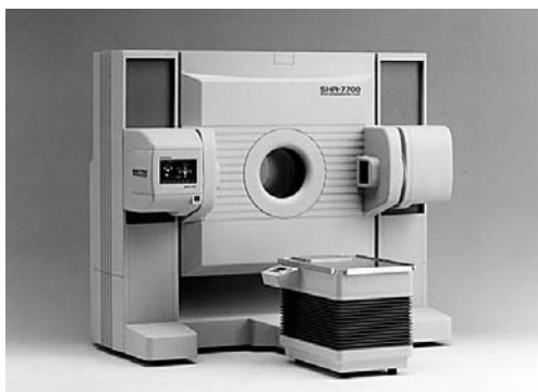
Figure 14-10: [Reference example] External view of Hamamatsu Photonics SHR-7700 PET scanner for animals
