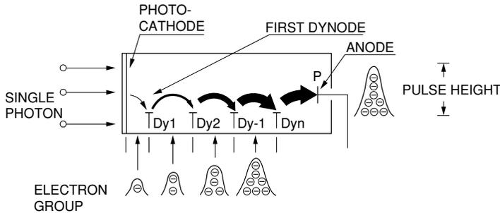
Figure 6-1: Photomultiplier tube operation in photon counting mode
