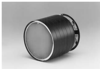
Figure 9-26: Grid type dynode photomultiplier tube
