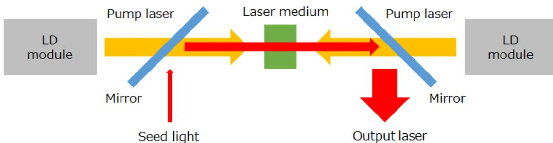
Schematic view of solid-state pulsed laser setup
