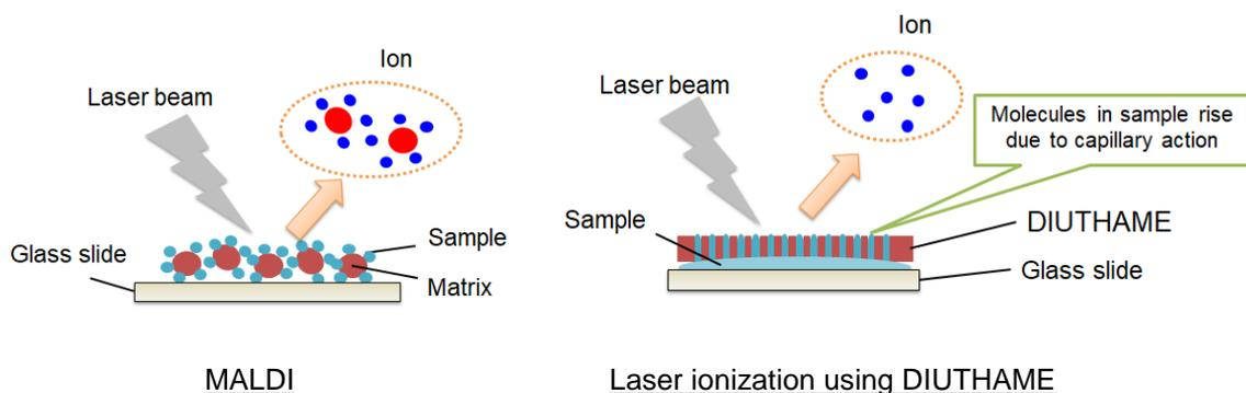
In the MALDI process, ionization occurs by laser irradiation on a sample pre-mixed with matrix.
