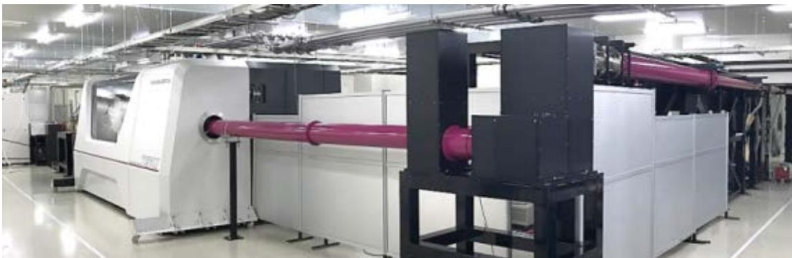
100-joule class laser (left in photo) and beam piping (purple pipes)
